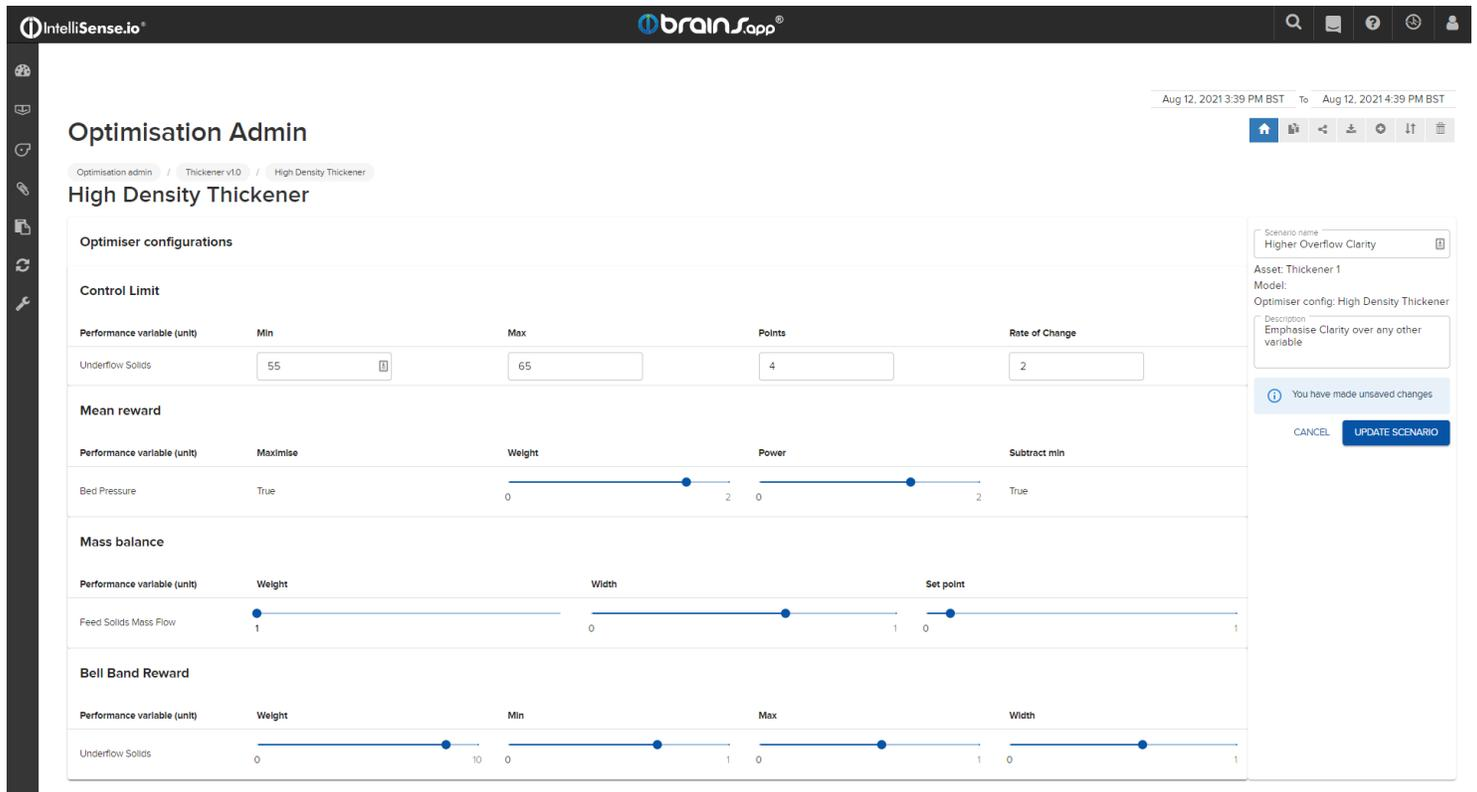
**Figure 5: Example of a Value Driver being configured for the Thickener Optimization Application.**
