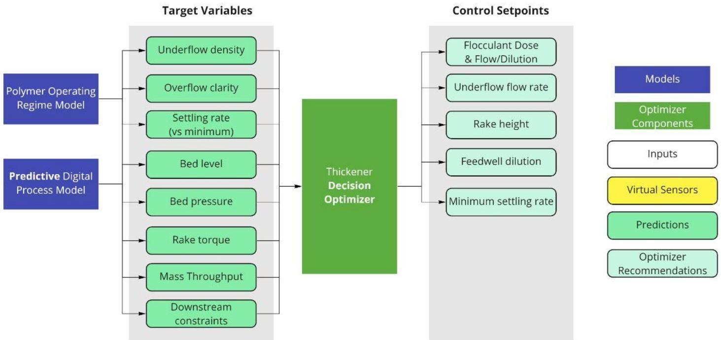
**Figure 7: The Predictions and Recommendations made by the Thickener Optimization Application.**
