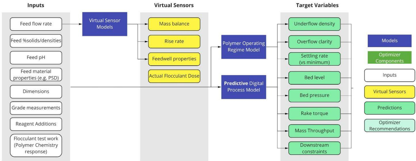
**Figure 4: Summary of the Thickener Optimization Application’s Inputs, Models, Virtual Sensors & Predictions.**
