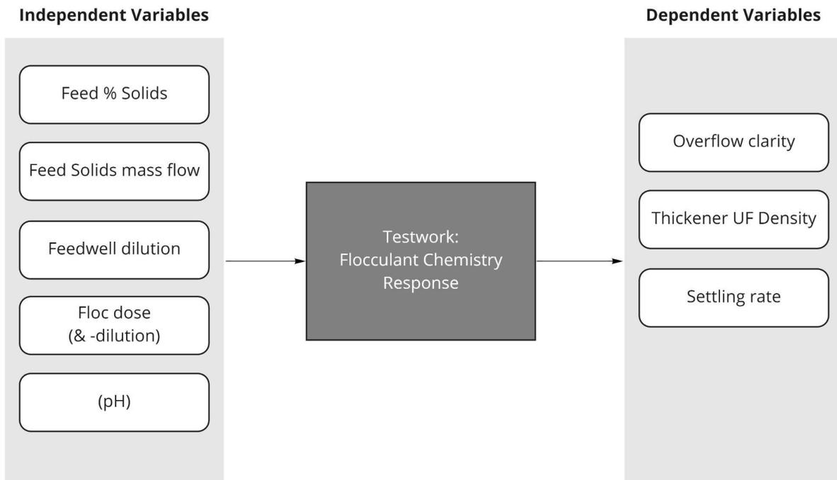
**Figure 1: Summary of key variables involved in BASF flocculant test work.**
