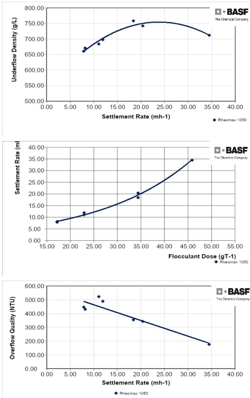
**Figure 2: Sample trends from BASF flocculant test work for a specific client.**
