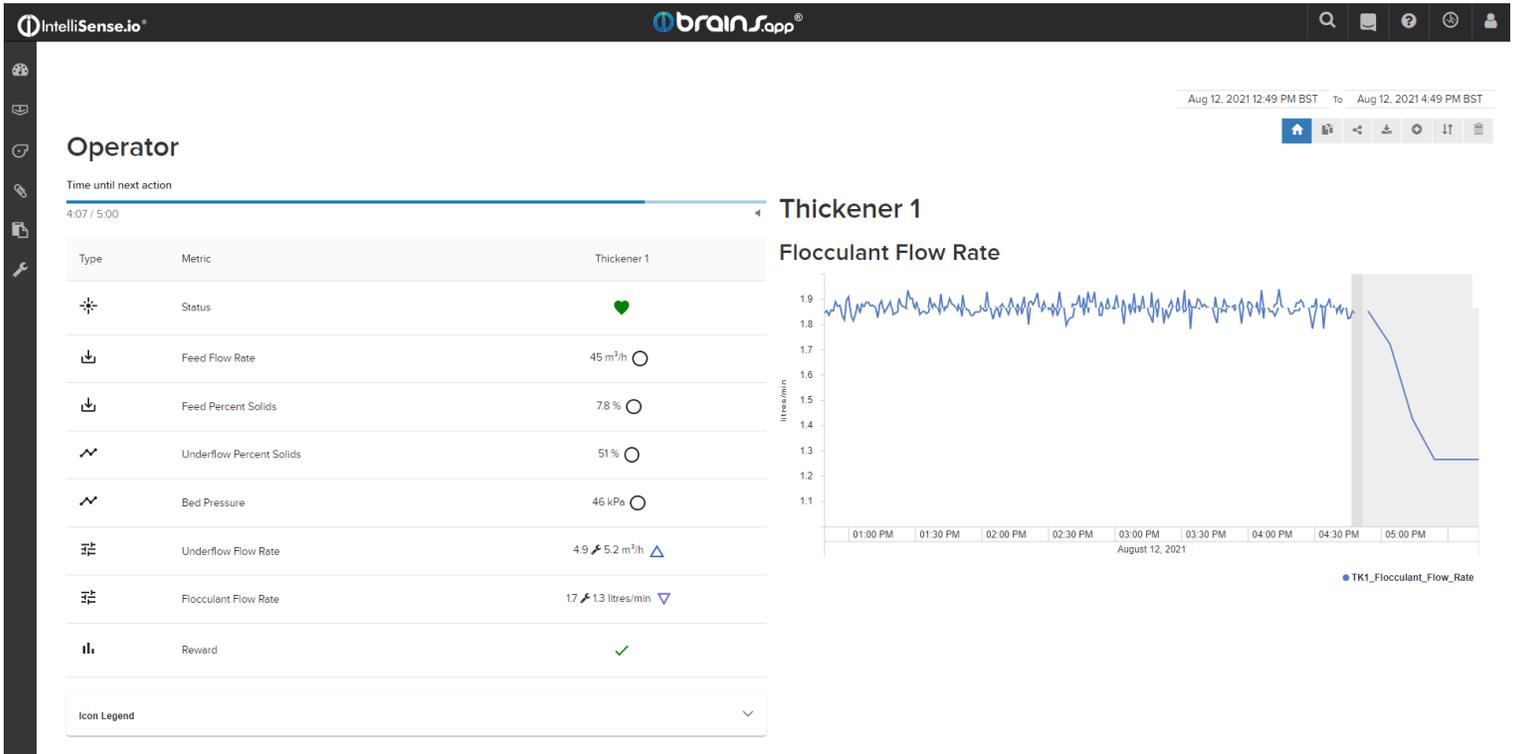
**Figure 6: Operator Screen, providing the Thickener Optimizer's recommendations to an operator as an advisory. The gray area on the right of the graph shows the recommended flocculant flow rate 60 minutes into the future.**
