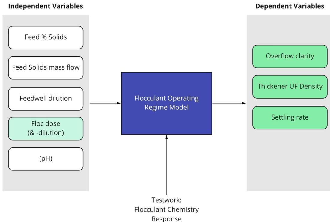
**Figure 3: Outline of the Flocculant Operating Regime Model, based on the test work.**
